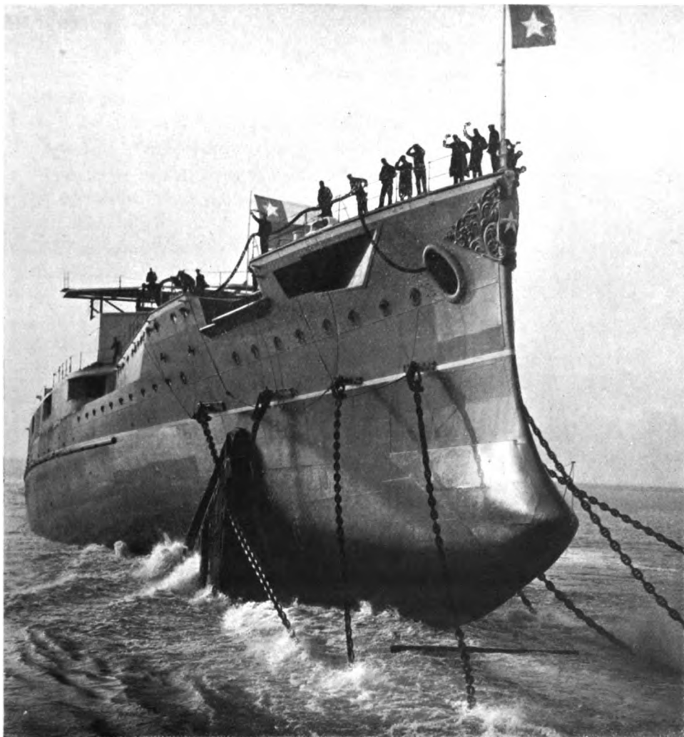
Launch of H.M.S. "Triumph," showing the unprotected area of a Battleship's Hull, below the water line.
