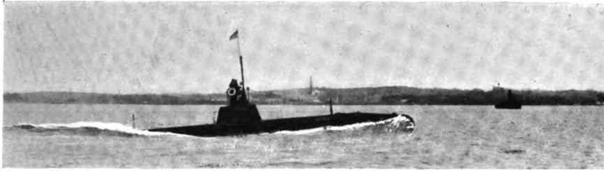
The U.S. Submarine "Octopus" running on the surface at 11 knots, light condition.
