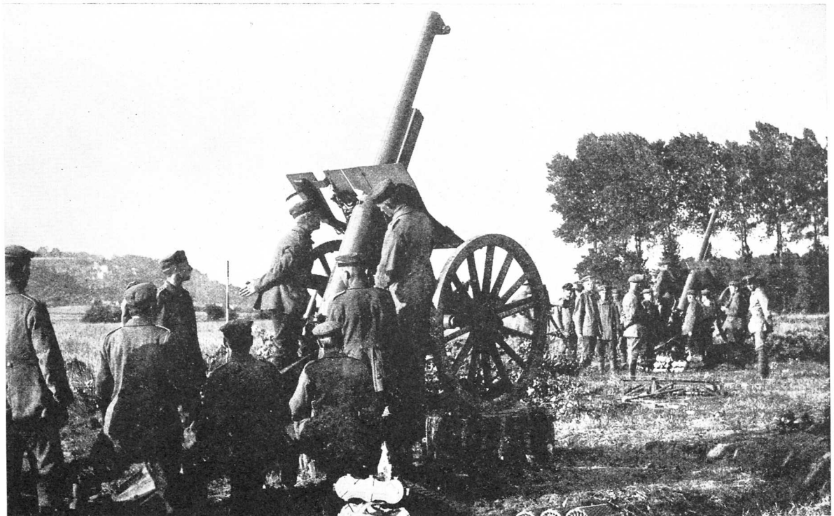
German aeroplane guns, mounted on turntables. They can be turned quickly to any direction and to whatever angle of elevation is required.
