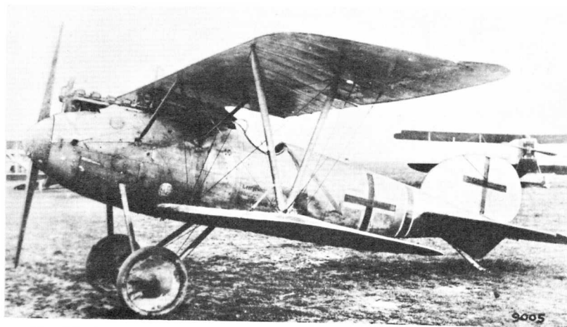
The Albatros D. Va was one of Germany's best WW I fighter planes. It carried 2 Spandau machine guns and had a speed of 116 MPH.
