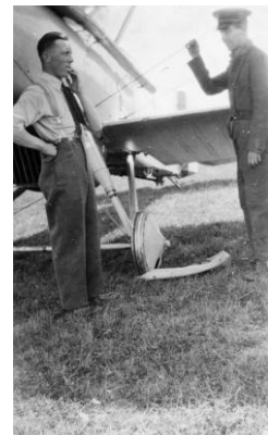
Figure 32. – Burst tyre at Upavon
